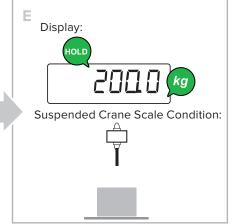
The weight remains displayed on the screen even when the scale is unloaded.
