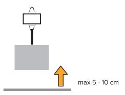
Weighing accuracy is achieved when the suspended crane scale is fully stationary.
