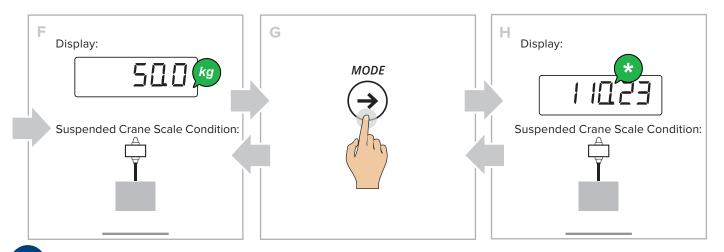
You can convert the unit of measurement with free conversion factor at any time by pressing  $\bigcirc$ .
