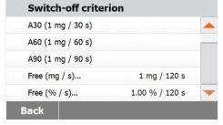
Select **Free (mg / s)** means weight loss per unit of time.
