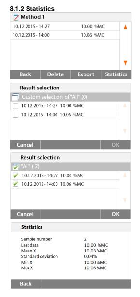
Select the method name to list all the test results of the method.
