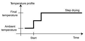
An alternate application possibility lies in the selective determination of the moisture at different temperatures. Gypsum, for example, releases only its surface water at 50°C,
