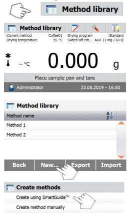
SmartGuide<sup>™</sup> helps you to find a method with optimal drying temperature automatically.
