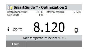
**Note:** The moisture analyzer needs to cool down if the temperature of heating chamber is above 40° C.
