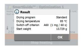
When the optimization process is finished, the **SmartGuide™** will provide an optimized heating method including drying program, drying temperate and switch-off criterion in the result.
