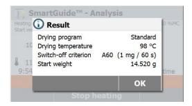
When the process is finished, the **SmartGuide<sup>TM</sup>** will provide a suggested heating method including drying program, drying temperature and switch-off criterion in the result.
