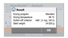
When the process is finished, the **SmartGuide<sup>TM</sup>** will provide a suggested heating method including drying program, drying temperate and switch-off criterion in the result.
