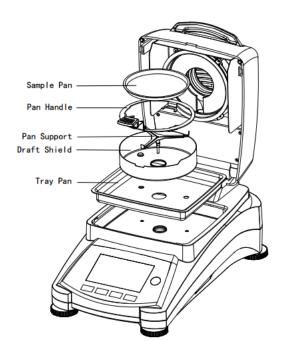
Open the cover and remove the pan handle, sample pan, draft shield, and heat shield from the instrument before cleaning.
