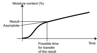
Measurement results of such a drying profile can be optimized:
