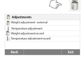
Press the Weight and temperature adjustment button to access adjustment menu.
