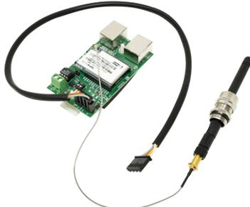
A green PCB with a white WiFi module and a long, flexible black antenna. A black square component is also visible on the board.                                                                       |
